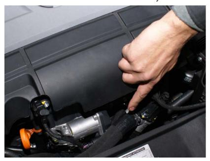
10) Remove torx screw holding N249 recirculation valve bracket.
