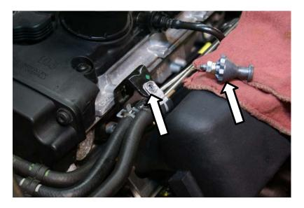
40) Trim notch in engine cover to provide clearance for oil dipstick and install engine cover. Add 2 inches of wire to intake air temperature sensor wiring with supplied butt connectors. After crimping connectors, please heat with heat gun or lighter to seal connections.
