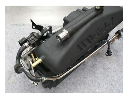
27) Retain the OEM flapper motor and trim down the flapper actuator arm as shown in the photo below so that it sits flush with the opening.
