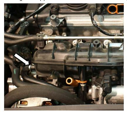
5) Remove both vacuum hoses from crankcase breather and valve cover.
