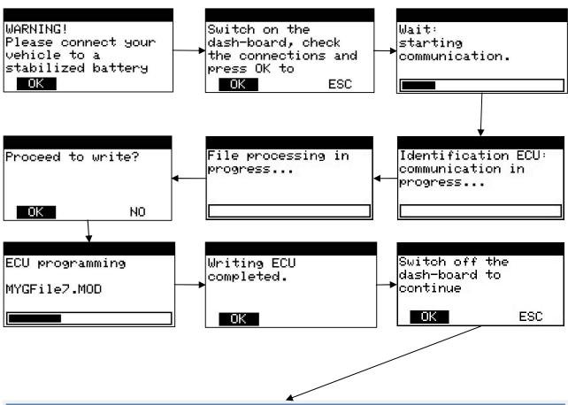
Click OK, switch off the dashboard and unplug the OBDII cable of the MyGenius from the car socket. Switch on the engine and verify that there are no warning lights on the dashboard. The car is now tuned with the modified file.
