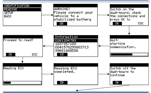
MyGenius tool has now properly read the ECU. Unplug the OBD II cable from the car and connect the USB cable to the MyGenius device and to the PC. To export the READING file from the device follow the instructions at pg.12 *file download* chapter.
