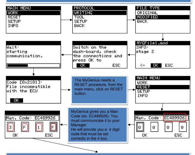
After click on OK button and MyGenius tool will be ready for a new automatic ID and reading on the vehicle with the new updated software version.
