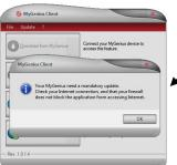
As soon as you receive the OK from the manager you can run the MyGenius software with the device connected via USB, the software will ask you to perform a mandatory update in order to download the specific command. At the end of the update the device will be ready to perform a new identification — reading procedure on the desired vehicle.
