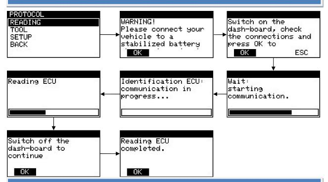
MyGenius tool has now properly read the ECU. Unplug the OBD II cable from the car and connect the USB cable to the MyGenius device and to the PC. To export the READING file from the device follow the instructions at pg.12 *file download* chapter.
