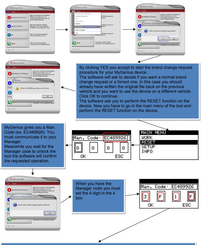
By clicking OK you can run the MyGenius software with the device connected via USB, the software will ask you to perform a mandatory update in order to download the specific command. At the end of the update the device will be ready to perform a new identification – reading procedure on the desired vehicle.
