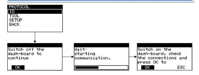
MyGenius tool has now properly identified the ECU. Unplug the OBD II cable from the car and connect the USB cable to the MyGenius device and to the PC.
