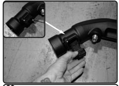
**29.** Install the MAF sensor into the new driver side tube. Secure and tighten using provided M4 screws.
