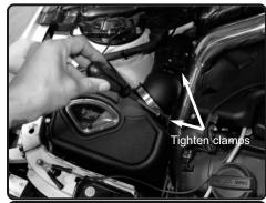
**20.** Install the tube to the Twist-Lock™ filter. Position for the best fit. Tighten both clamps using 8mm nut driver.
