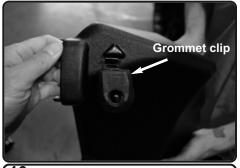
**16.** Locate the factory grommet clip that holds in factory air box located on vehicle frame. This will be used to secure new injen air box. Now install the grommet to the injen airbox fitting and secure.
