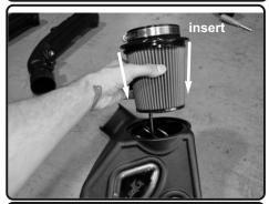
**31.** Position the Twist-Lock™ filter pattern to the hole cut out on air box.
