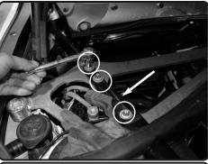
**6.** Loosen the 3 bolts on the end of the strut bar and remove. Continue on other side.
