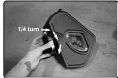
**15.** Now secure the Twist-Lock™ filter turning 1/4 turn in either direction. Make sure the filter locks into place. *Please note clear windows not available.*
