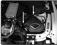
**28.** Now install the driver side air box into the vehicle and secure. Make sure fitting on air box are secured in grommet.
