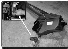
**27.** Remove the grommet clip from OEM air box.
