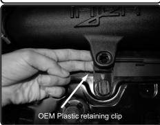
**31.** Reuse a OEM plastic retaining clip to secure the front of the Injen tube to the bracket.
