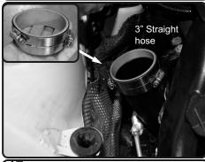
17. Place clamps to 3" hose like above image for easy access when securing the clamps. Now install the hose assembly to the turbo housing. Tighten the clamp on the housing only using 8mm nut driver.
