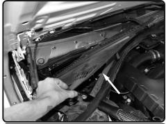
**3.** Loosen the engine tray and pull back weather trim seal.
