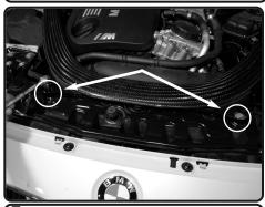
**7.** Now loosen the 2 bolts holding in the front of the strut bar on the radiator support.
