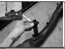
**26.** With t25 torx bit, loosen the 2 screws holding in the MAF sensor. Carefully remove the MAF sensor.
