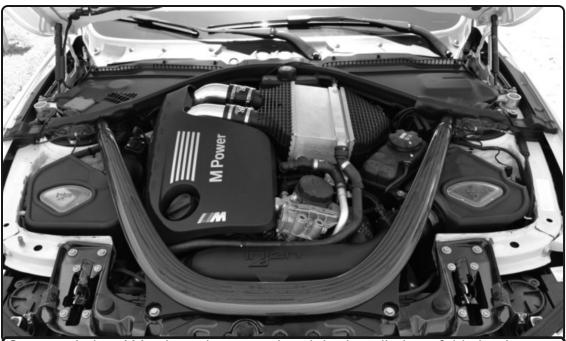
Congratulations! You have just completed the installation of this intake system. Periodically, check the alignment of the intake, normal wear and tear can cause nuts and bolts to come loose. <u>Note: Check clearance and adjust if needed! Failure to check the alignment and adjust the intake can cause damage that will void the warranty. Injen Technology is not responsible for any damages caused by/from improper installation.
