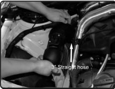
**18.** Install the passenger side intake tube and position Do not tighten clamp
