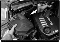
**10.** Pull back the intake hose, now lift up and remove the passenger side air box out of vehicle.
