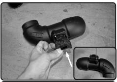
**13.** Install the MAF sensor into the passenger side intake tube. Secure and tighten using provided M4 button head screws.
