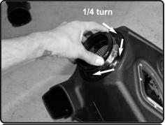
**32.** Now secure the Twist-Lock™ filter turning 1/4 turn in either direction. Make sure the filter locks into place.
