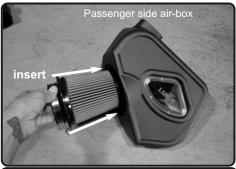
**14.** Install the filter into the passenger side air box housing. Position the Twist-Lock™ filter pattern to the hole cut out on air box. *Please note clear windows not available.*
