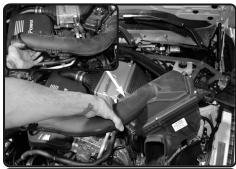
**25.** Now lift up and remove the driver side intake system out of the vehicle.
