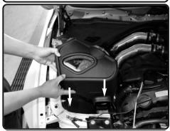
**19.** Now install the passenger side air box into the vehicle and secure. Make sure fitting on air box are secured in grommet. Make sure clip from step 16 is secured to frame.
