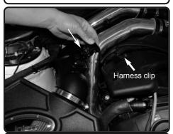
**21.** Pull back the harness clip from the engine cover. Now connect the MAF sensor. Verify passenger side is secured and clamps are tight.
