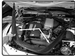
**8.** Now lift up and remove the factory strut bar. This will now have access for the intake systems.
